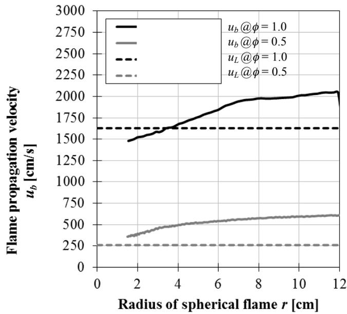
Fig.3 Profile of flame propagation velocity at  $\phi = 1.0$
