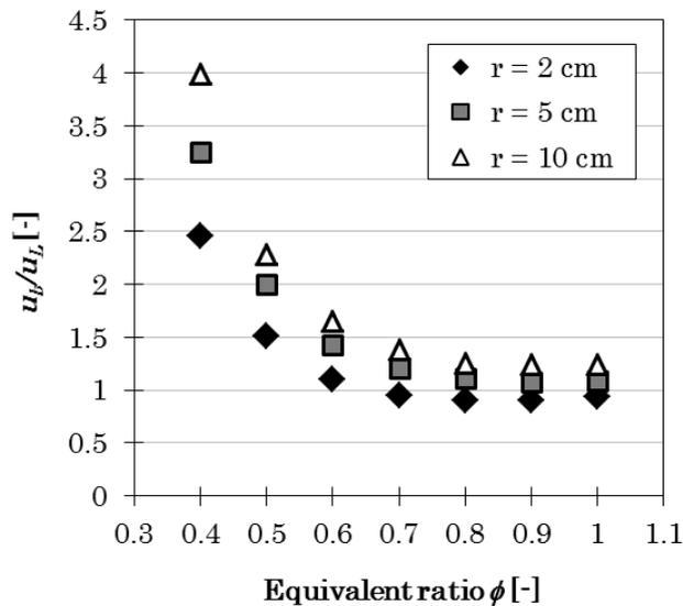
Fig.4 Ratio of experimental propagation velocity to calculated propagation velocity
