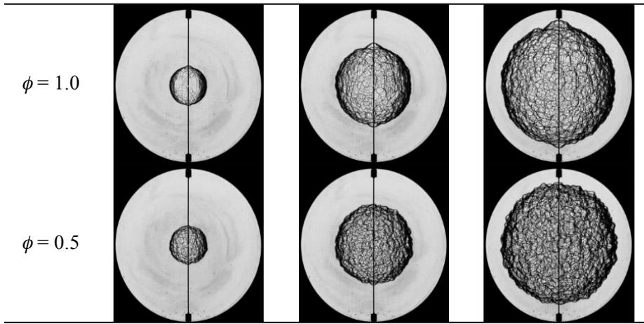
Fig.2 Schlieren photograph at  $\phi = 1.0$  and  $0.5$
