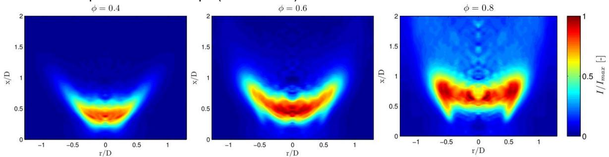
Figure 5: Abel-deconvoluted time-averaged  $OH^*$  images normalized by maximum intensity of  $\phi=1$ , indicating location of heat release. Images recorded at a mass flow of 180 kg/h and an inlet temperature of 620 K for configuration with long mixing tube and high swirl.
