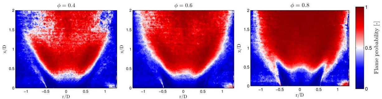
Figure 4: Flame probability indicating the location of maximum flame front likelihood, thus, allowing to determine the upstream flame shape ( $Re = 75\,000$ ).
