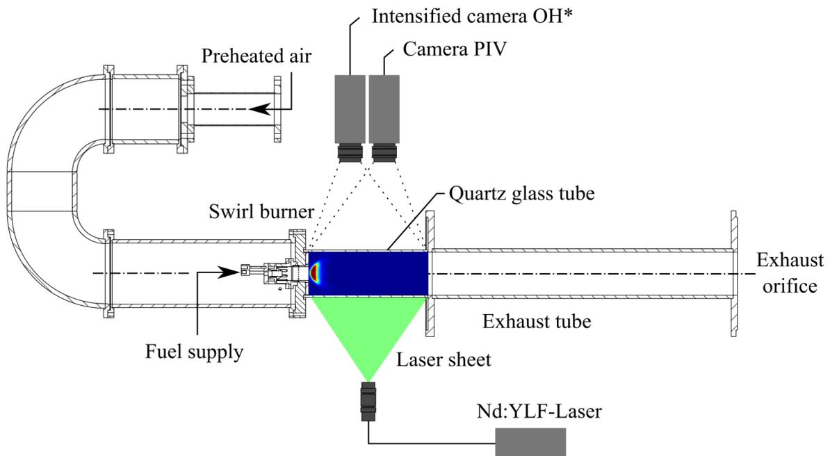
Figure 2: Schematic of the experimental setup for gas-fired atmospheric tests applying high-speed PIV and  $OH^*$  imaging
