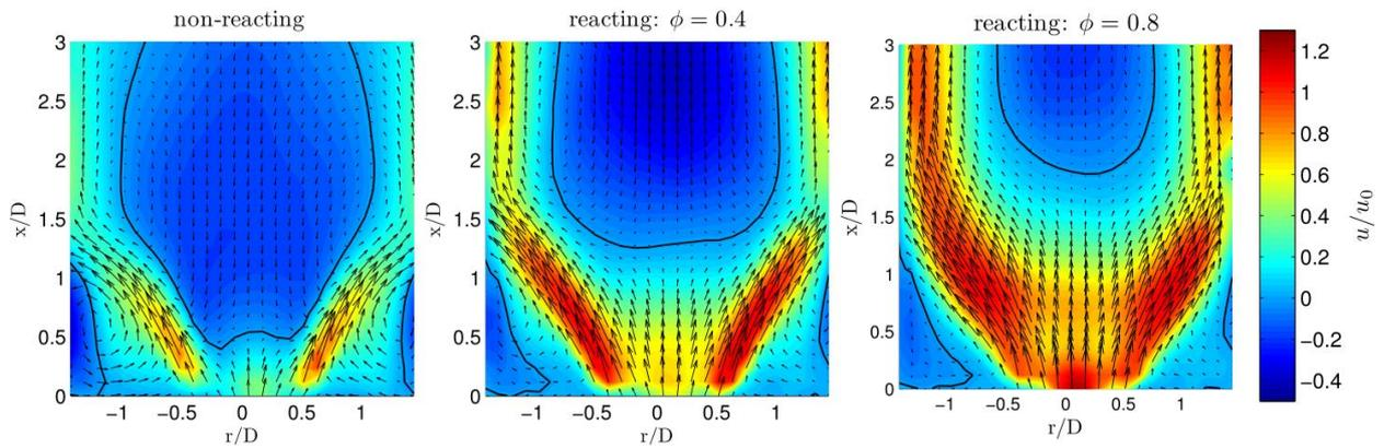
Figure 3: Time-averaged velocity vectors superimposed on the normalized axial velocity to visualize the impact of equivalence ratio on the flow field.
