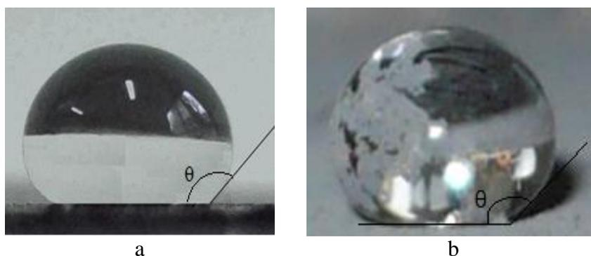
Fig. 4. The behavior of water droplets placed on the surface of a quartz plate coated with a layer of hydrophobic soot: a - drop of water on the superhydrophobic carbon during combustion propane with a nickel catalyst; b - water drop on surface soot obtained during combustion of pyrolysis products of polyethylene waste with a nickel catalyst.
