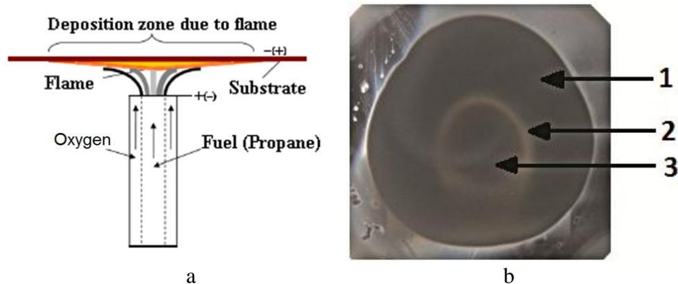
Fig. 1. Scheme of installation and a photograph of the substrate: a) schematic illustration of burner device; b) a silicon disk with a hydrophobic coating at 4 min exposure to a propane/oxygen flame with flow rate 150/310 cm<sup>3</sup>/min, showing of three deposition zones.
