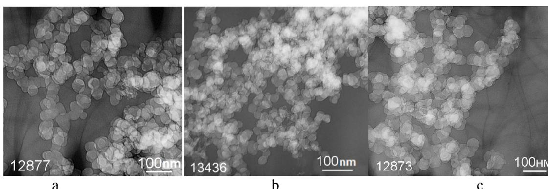
Fig. 5. Electron micrographs of soot during combustion products of the catalytic pyrolysis of plastic waste a) without additional influences; b) with an applied electric field 1 kV; c) with a nickel catalyst
