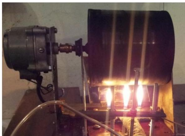
Fig. 3. Image of the experimental installation for synthesis superhydrophobic carbon black during combustion of pyrolysis products of polyethylene waste
