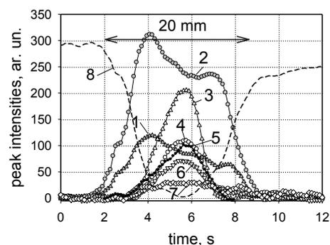
Fig. 2. Dependences of peak intensities on time, measured by a probe at the 0.6 mm distance from the pine needle 1-  $I_{18}/10$  ( $H_2O$ ), 2 -  $I_{44}/10$  ( $CO_2$ ), 3-  $I_{31}$ (ethanol, butanol), 4, 6 -  $I_{60}$ ,  $I_{73}$  (levoglucosan), 5 -  $I_{68}$  (furan), 7 -  $I_{58}$  (acetone), 8 -  $I_{32}/15$  ( $O_2$ ).
