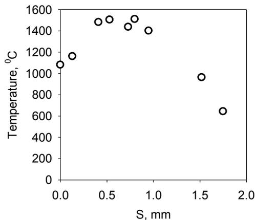
Fig. 6. A temperature profile of the flame perpendicular to the SPN in the location of the maximum temperature of the SPN
