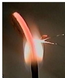
Fig. 5. A photo of the flame when spread down a vertically positioned SPN and of a thermocouple
