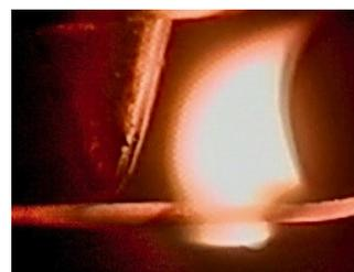
Fig. 1. Photo of flame spread across a single pine needle, the probe is to the left of the flame.
