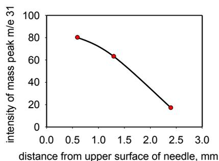
Fig. 4. Dependence of the intensity of mass peak 31 on the distance from the upper surface of the burning SPN
