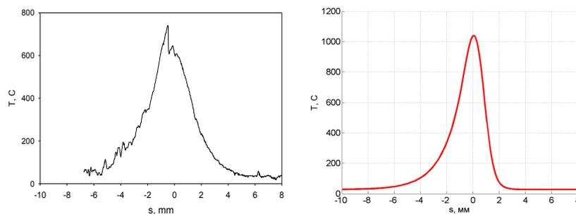
Fig.7. Temperature profiles: measured with a thermocouple (left) and calculated (right).
