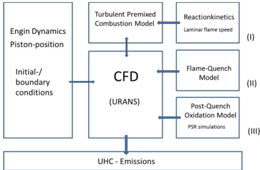
**Figure 1:** Schematic of the Hybrid-Model
