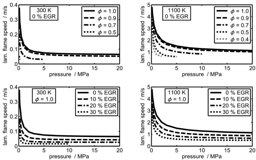
**Figure 2:** Laminar flame speed of methane-air-mixtures from reaction kinetic calculations within a pressure range of 0.1 to 20 MPa for unburned gas temperatures of 300 and 1100 K, shown for varying equivalence ratios (top) and EGR rates (bottom).
